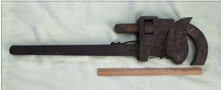
The photograph above shows the prototype of Rufus F. Boop’s invention - the Perfection Pipe Wrench. This wrench is owned by Neil and Alice Shoreman of Millmont.
